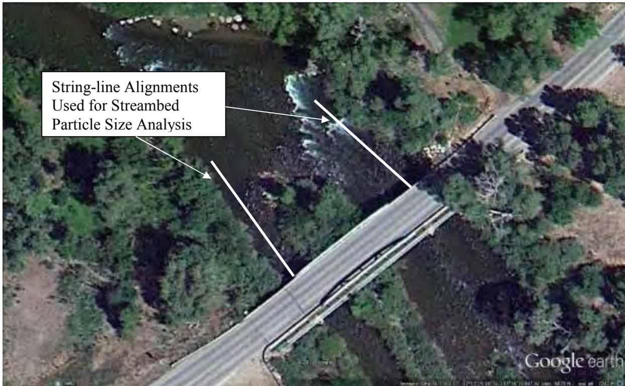
Based on our field measurements, a  $D_{50}$  particle size of about eight (8) inches was calculated for the main channel streambed surface particles. The smallest particle size measured was about three-quarter ( $3/4$ ) inch in diameter while the largest particle size measured was about sixteen (16) inches in diameter.
